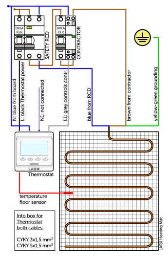
Note: Outputs marking is valid for LARX LCD Thermostat. For other thermostats check their manual.
